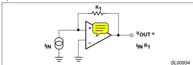
Figure 4. Current-to-Voltage Converter
