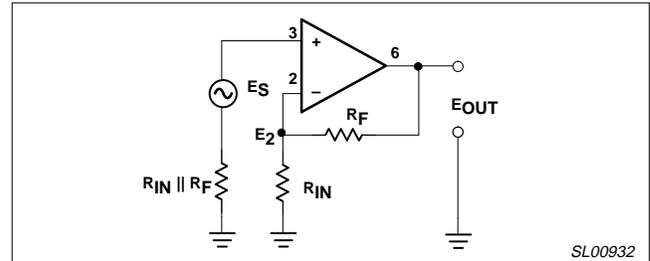
Figure 2. Non-Inverting Amplifier
