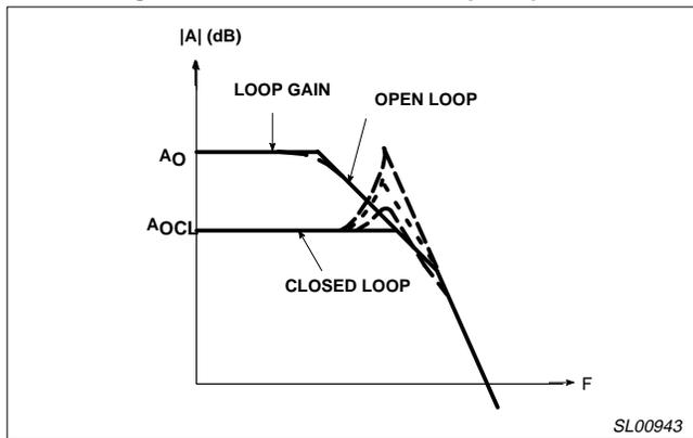
Figure 13. Frequency Peaking Due to Insufficient Phase Margin
