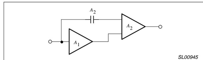
Figure 15. Technique of Feed-Forward Around 1st Stage
