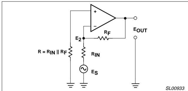
Figure 3. Inverting Amplifier
